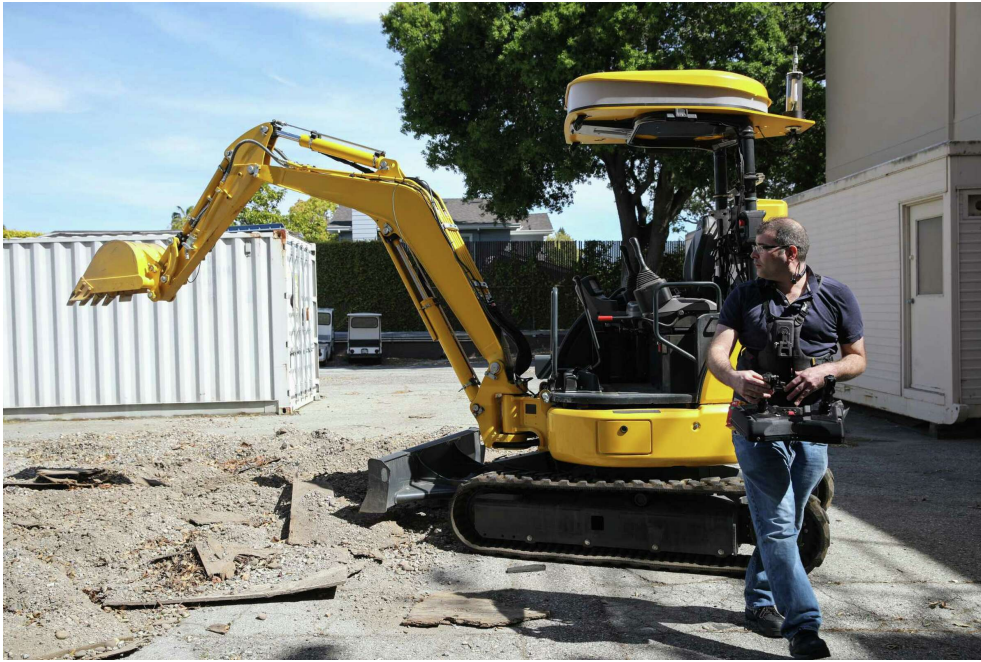
Senior Robotics Researcher Reuben Brewer remotely operates SRI International's Internet Remote Controlled Excavator at the SRI campus. Juliana Yamada/The Chronicle
