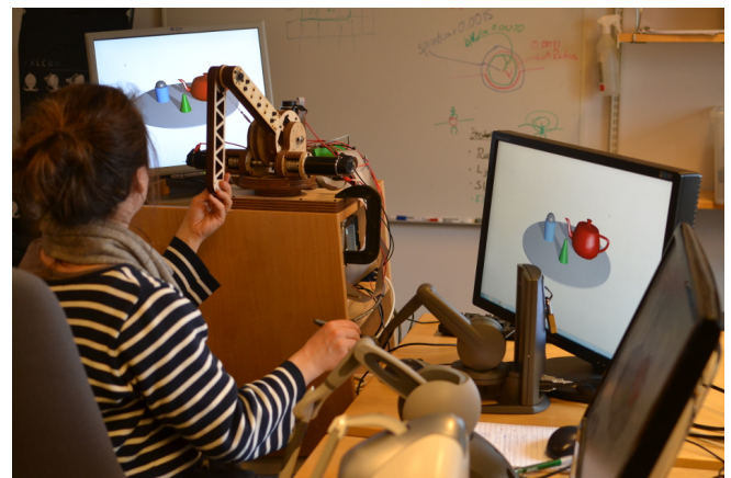
Figure 9. The setup of the evaluation showing the four different devices and the demo application used in the test.
